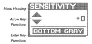
All menus use the same general layout as shown in the sample menu. The heading of the menu is at the top. The area in the center is controlled by the UP and DOWN arrows, and the area under the horizontal line is controlled by the ENTER button. Not all menus are affected by all controls, but the layout is the same regardless. Pressing MENU repeatedly will sequentially display all available menus.
